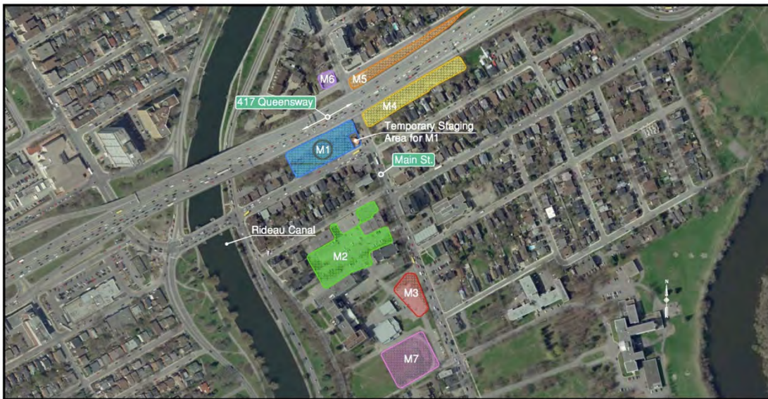
POTENTIAL STAGING SITES FOR MAIN STREET BRIDGE
