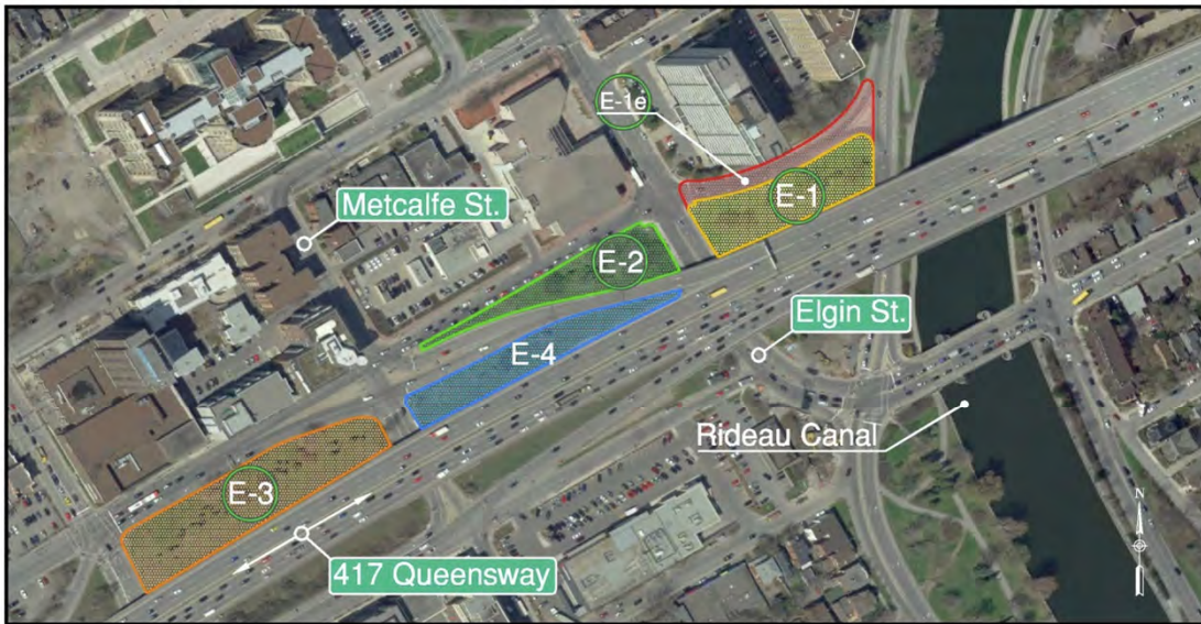
POTENTIAL STAGING SITES FOR THE METCALFE STREET AND ELGIN STREET BRIDGES
